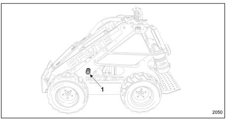
Figure 4-16 Clean Spark Arrestor
